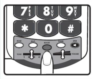
The BOOST button controls the loudness of the receiver. Once the BOOST button is pressed, an extra level of amplification is added over the entire range of the Volume Control.
